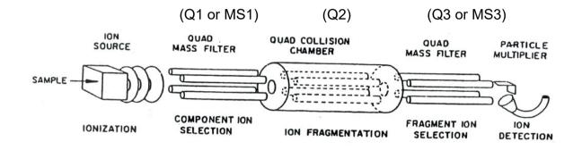
The machine is divided in five parts: the ion source where the ionization takes place; the first mass analyzer (Q1 or MS1) for component ion selection; the quad (quadrupole) collision chamber (Q2) where ion fragmentation by CID is performed; the second mass analyzer (Q3 or MS2) for fragment ion selection; and the particle multiplier for ion detection.
