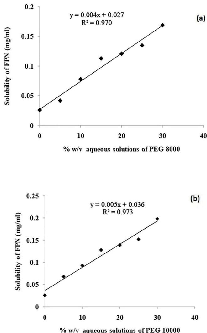
**FIGURE 1** - Phase solubility curves of FPN in aqueous solution of PEGs at 25 °C (n=3) [(a) in PEG 8000, (b) in PEG 10000].
