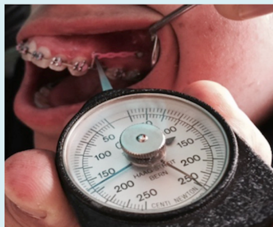
Figure 2. Measurement of force by the orthodontic gauge.
