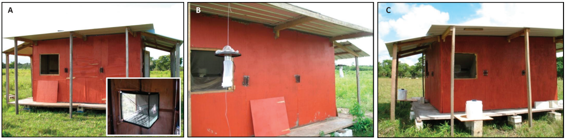
Fig. 2. (A) An experimental hut at the field site with an open window (portal for mosquito entry), with a window interception trap used to monitor mosquito entry (inset). (B) Baited Centers for Disease Control and Prevention light traps and (C) baited BG-Sentinel™ traps positioned outside each portal of entry.
