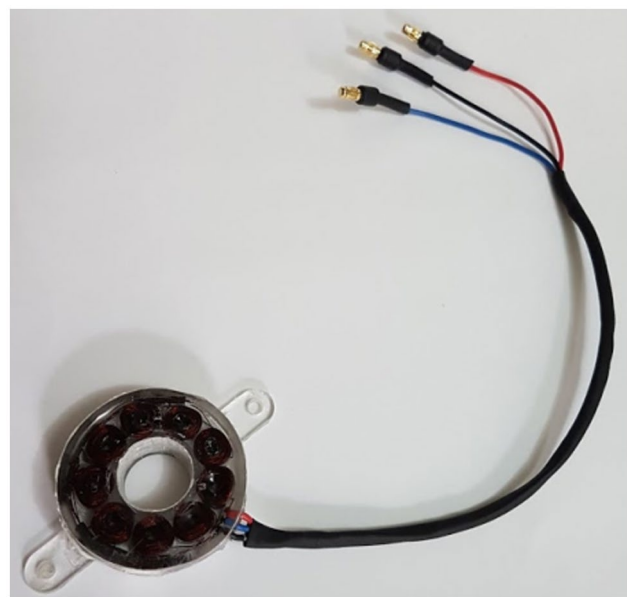
FIGURE 6 Complete stator with wires and terminals [Color figure can be viewed at wileyonlinelibrary.com ]
