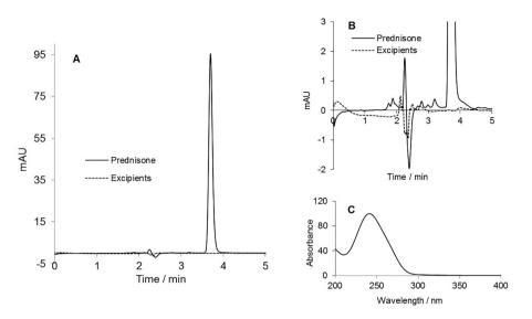
**FIGURE 3** - (A) Chromatograms of prednisone reference standard at 14.0  $\mu$ g mL<sup>-1</sup> and placebo sample using the optimized conditions of the chromatographic method. (B) Expanded chromatograms of (A). (C) Spectrum of ultraviolet absorbance in the range 200-400 nm for prednisone.
