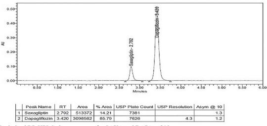
FIGURE 7 - Optimized RP-HPLC chromatogram for SAXA and DAPA at 210 nm
