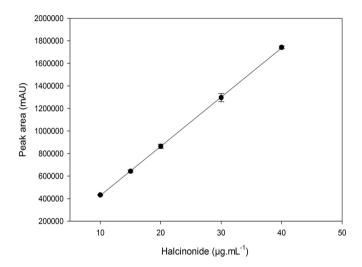
**FIGURE 3** - Mean calibration curve obtained to halcinonide using working standard solutions at the concentration range from 10.0 to  $40.0 \ \mu g.mL^{-1}$  (n=3).
