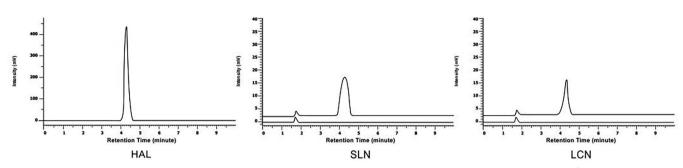
**FIGURE 2** - Representative HPLC chromatograms obtained from halcinonide standard solution (25.0  $\mu$ g.mL<sup>-1</sup>) in methanol:water and halcinonide-loaded and unloaded nanoparticles: LCN and SLN. Mobile phase: methanol:water (85:15 v/v); flow rate: 1.0 mL/min; detection wavelength: 239 nm; column temperature: 25±2 °C; and injection volume: 20  $\mu$ L. HAL: halcinonide. Retention time: 4.21 minutes.
