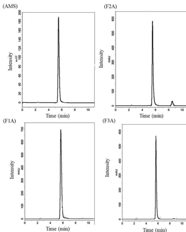
**FIGURE 2** – HPLC chromatograms of AMP, F1A, F2A and F3A by UV detection.
