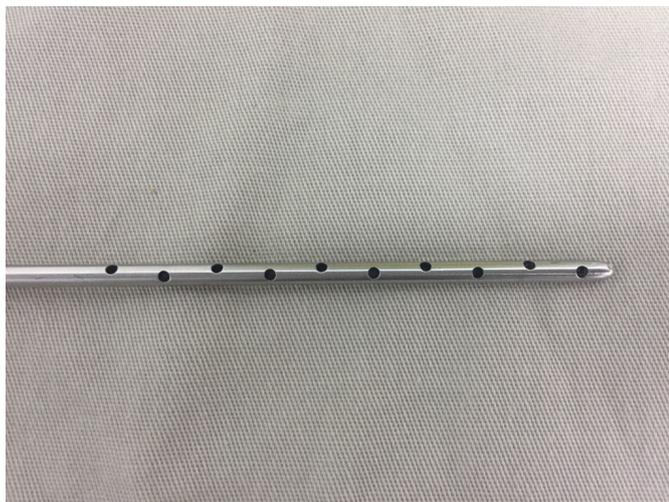
**Figure 1.** Detail of the design and arrangement of the orifices of the 10-hole cannula prototype.
