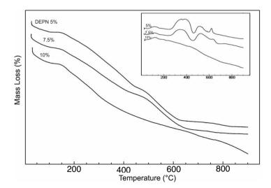
**FIGURE 2** - Thermogravimetry (TG) and DTG of the DEPN 5%, 7.5% and 10% extractive solutions in nitrogen atmosphere (50 mL·min<sup>-1</sup>) and a heating rate of 10 °C min<sup>-1</sup>.
