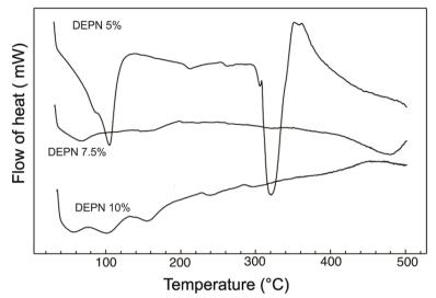
**FIGURE 1** - Differential scanning calorimetry (DSC) of the DEPN 5%, 7.5% and 10% extractive solutions in a synthetic air atmosphere (50 mL·min<sup>-1</sup>) at a heating rate of 10 °C min<sup>-1</sup>.
