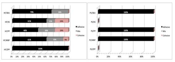
Figure 4. Fracture Mode Analysis after 3 months.
