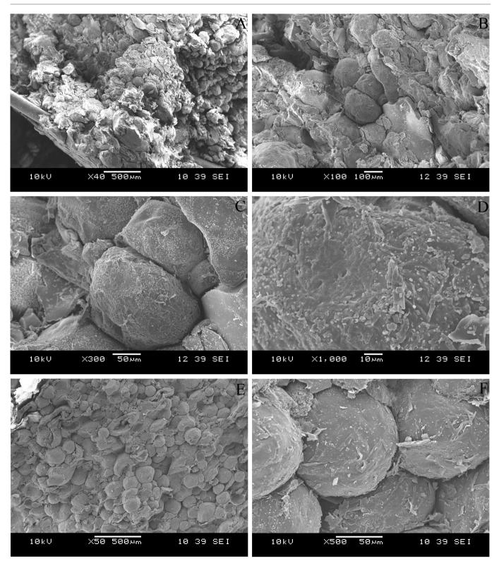
**FIGURE 3** – Scanning electron micrographs of tablets made with PIP-MP and adjuvants (PIP-MP-T) with magnification of 40x (A), 100x (B), 300x (C) and 1000x (D) and only with PIP-MP (PIP-MP-Tnd) with magnification of 50x (E) and 500x (F).
