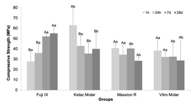
Figure 1 – Compressive strength (MPa) and standard deviation of conventional glass ionomer cements evaluated in time interval up to 28 days. Different uppercase letters indicate statistically significant differences within the same material, and different lowercase letters indicate statistically significant differences within the same time interval (p<0.05).
