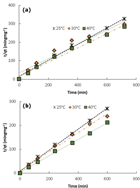
Figure 6. Kinetic model pseudo-second order for the adsorption of DB-86 dye at different temperatures: a) CAM and b) CAY.
