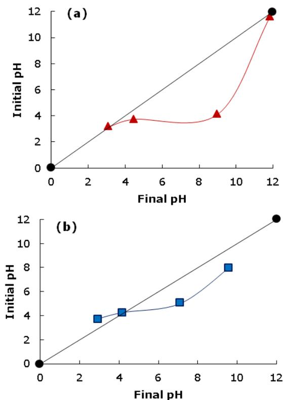
**Figure 2.** Point of zero charge of CAY (a) and CAM (b).
