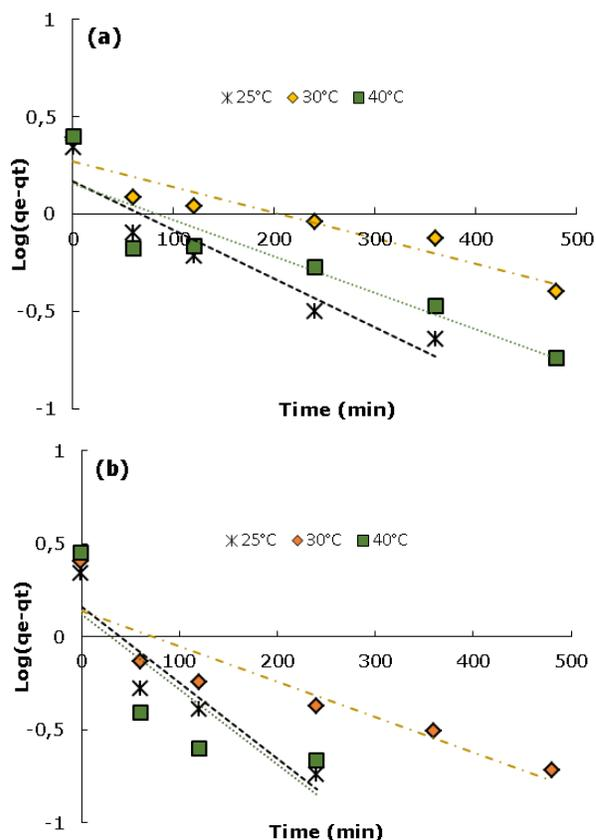
Figure 5. Kinetic model pseudo-first order for the adsorption of DB-86 dye at different temperatures: a) CAM and b) CAY.
