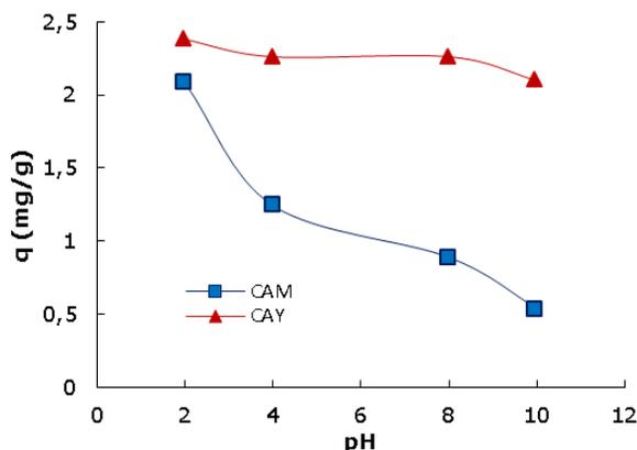
Figure 3. Effect of pH on the maximum capacity of adsorption.
