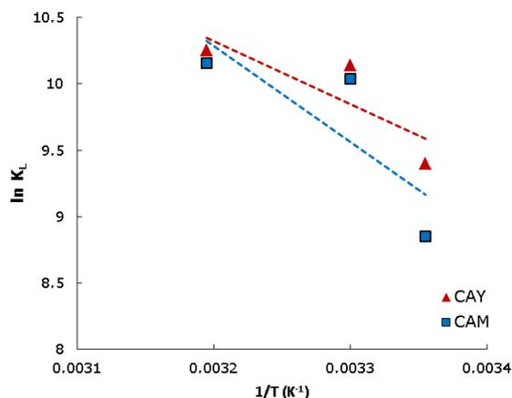
Figure 4. Thermodynamics of the adsorption of DB-86 dye on activated carbons CAY and CAM at pH 2.
