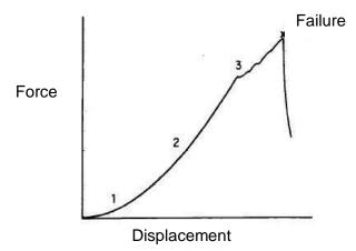
Figure 2 - Tendon load-deformation Curve. (1) toe region; (2) linear region; (3) yield region.
