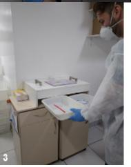
**Figure 1.** "UVC box" for disinfection of supplies returned to the pharmacy: portable device at different angles (1, 2 and 3) with two 18W lamps each.
