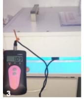
**Figure 3.** Different angles (1, 2 and 3) of the radiometer used to measure the power and radiation dose of the "UVC box": essential for full control of the use of lamps.
