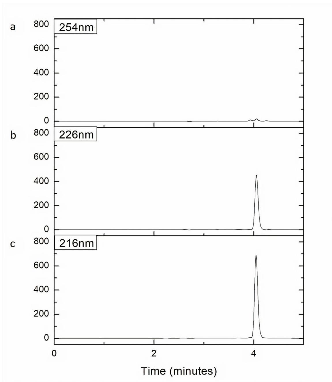
**FIGURE 2** - HPLC chromatogram of 100  $\mu\text{g/mL}$  standard ACA solution at UV detection wavelengths of a) 254 nm, b) 226 nm and c) 216 nm. Conditions: mobile phase acetonitrile:water ratio of 80:20 (v/v), flow rate of 0.8 mL/min, column temperature of 25 °C, sample temperature of 25 °C, and injection volume of 10  $\mu\text{L}$ .
