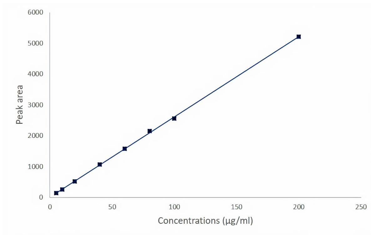
**FIGURE 4** - Mean calibration curve of standard ACA solutions at concentrations ranging from 5 to 200 µg/mL (n=3)
