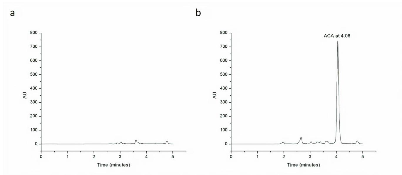
**FIGURE 3** - HPLC chromatograms of a) precipitate from blank NLCs and b) precipitate from ACA-NLCs. Conditions: mobile phase acetonitrile:water ratio of 80:20 (v/v), flow rate of 0.8 mL/min, column temperature of 25 °C, sample temperature of 25 °C, and injection volume of 10  $\mu$ L.
