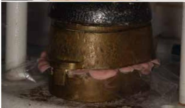
**Fig. 4.** Excess acrylic flash after trial pack.
