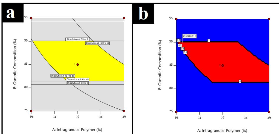
**FIGURE 6 - a)** Optimized design space for independent variables A and B; **b)** Desirability plot for independent variables.
