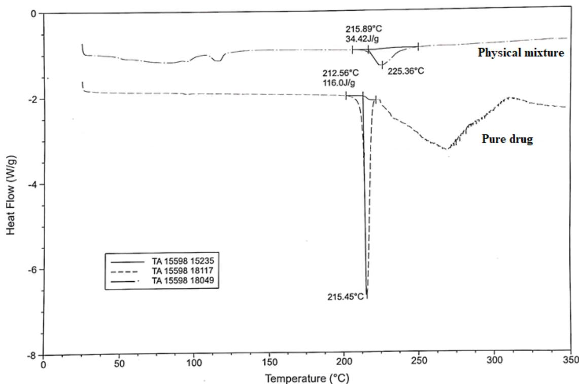
**FIGURE 3** - DSC thermograms of pure drug and Physical Mixture.
